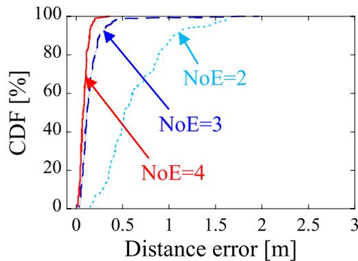
Fig. 15 CDF of distance error with various numbers of antenna elements.
