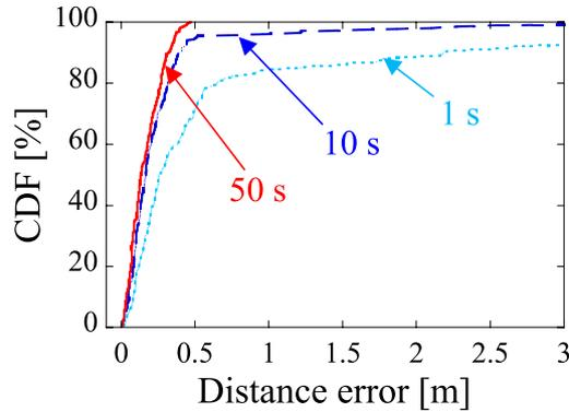
Fig. 14 CDF of distance error with various channel measurement periods.
