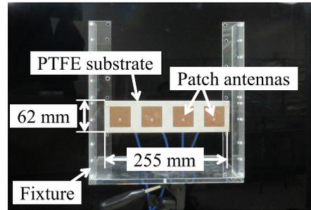
**Fig. 2** Measurement system.
