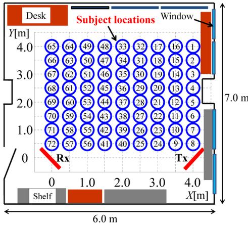
Fig. 3 Measurement environment.
