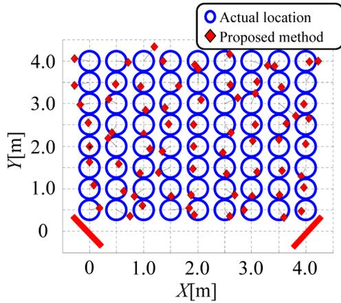
**Fig. 7** Localization results from 72 measurement positions when a single target was present.
