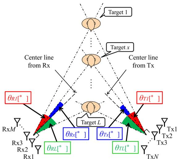
Fig. 1 Concept of living-body localization method.
