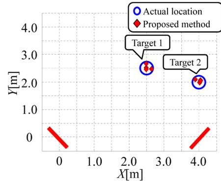
(b) Two target directions are not overlapped from either antenna.
