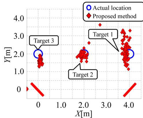
**Fig. 9** Localization accuracy results from 100 trials when three targets were present.
