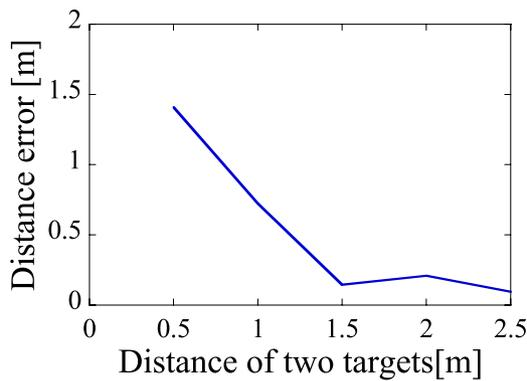
Fig. 11 Distance error with two targets separated by various distances.
